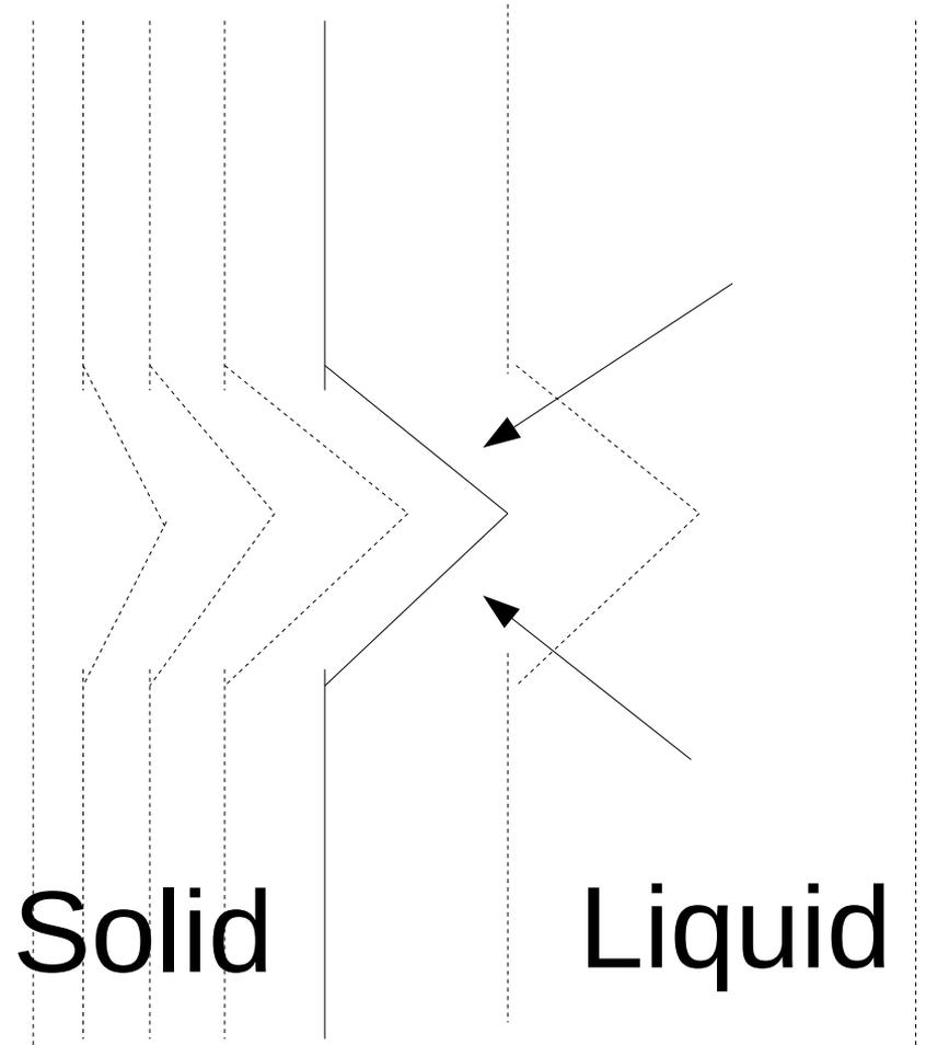
Broken lines: isothermal (lines of same temperature); arrows: direction of heat flow
