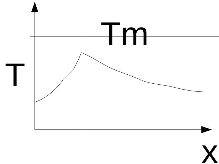
Let us consider a supercooled melt, from which, the heat is removed on one side. In such a case, sometimes, a temperature profile as shown can develop. This is known as temperature inversion.
